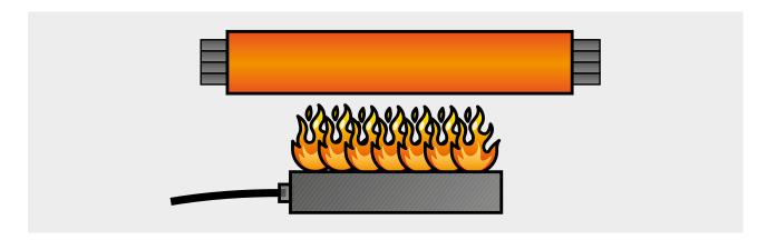
Cables satisfying the requirements of this type of standard are manufactured using materials such as fibre glass, fire-proofed components with polyolephine, silicone or fluorinated polymers. (IEC 331-23 cable)
