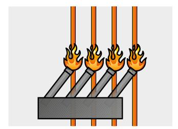
The tests according to IEC 60332-3 comprise 4 test categories (A - B - C - D) according to the volume of combustible material per metre of cable.
