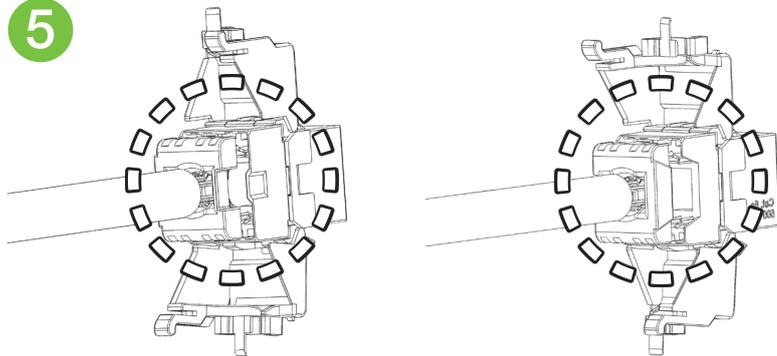
Place wiring insert in the keystone housing
