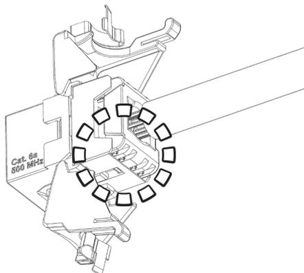
Make sure that the wiring cap is correctly insert in the body
