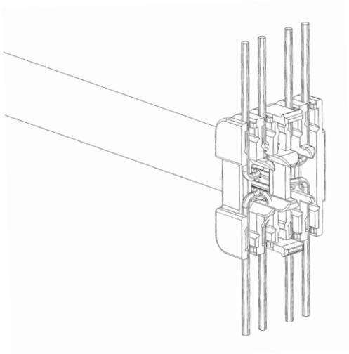
Separate the wires according to colour coding.
