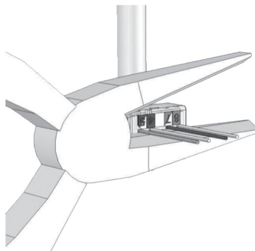
Cut the wires excessive length.
