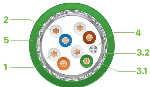
1. **Conductor** : solid bare copper AWG26/7
