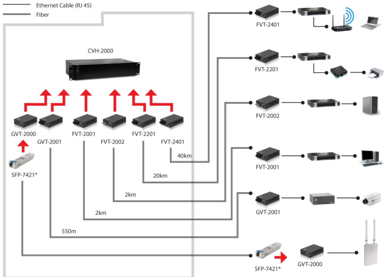
\*In above example diagram, converter modules at local and remote ends should be paired for proper connectivity, and the distance mainly depends on cable and transceiver selection accordingly.
