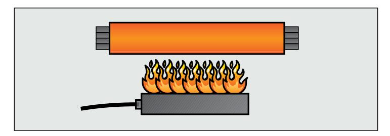
Cables satisfying the requirements of this type of standard are manufactured using materials such as fibre glass, fire-proofed components with polyolephine, silicone or fluorinated polymers. (IEC 331-23 cable)
