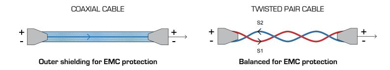
Given today's throughputs, a non-shielded twisted pair cable would seem to be an effective response to bandwidth requirements. The arrival of the 1000 BASE T and, in particular, the 10G BASE T with more sensitive encoding will lead to us favouring shielded options.
