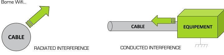
This interference is a characteristic of inductive or capacitive electrical phemomena associated with the performance of the products used and the quality of a system's installation. Regulatory documents are available on this topic which govern the entire scope of EMC
