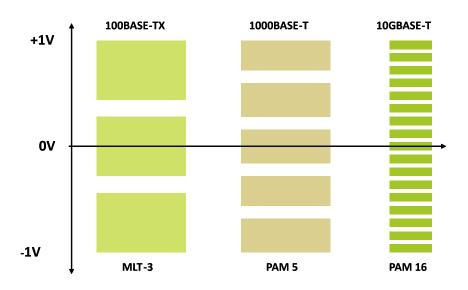
Thanks to increasingly more sensitive encoding, the noise level acceptable for today's networks is 100 times greater than before. Electromagnetic immunity is becoming fundamental.v
