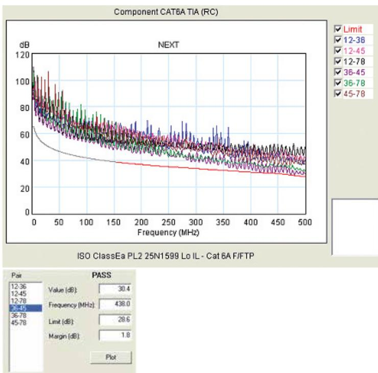
The same link is re-certified in accordance with the ISO Class Ea (Low IL because link is in progress)
