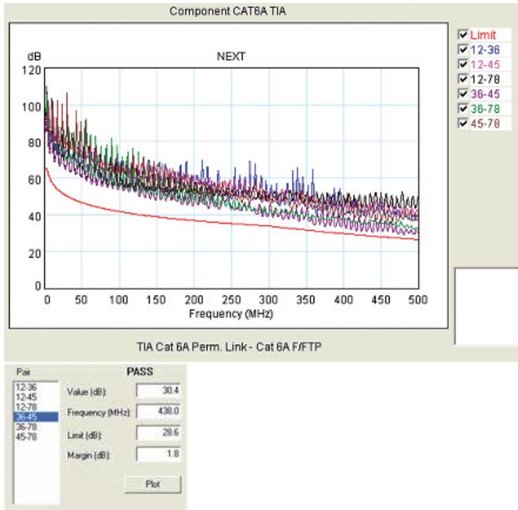
Measurement performed on an 18 meter link with commercially available TIA Cat6A components.
