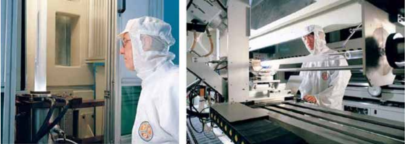
Manufacturing a preform in our TFO plant in Nanjing.
