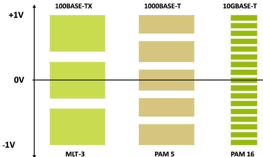
Thanks to increasingly more sensitive encoding, the noise level acceptable for today's networks is 100 times greater than before. Electromagnetic immunity is becoming fundamental.
