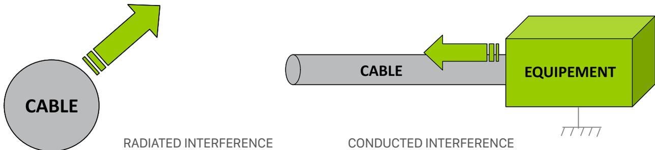
This interference is a characteristic of inductive or capacitive electrical phenomena associated with the performance of the products used and the quality of a system's installation. Regulatory documents are available on this topic which govern the entire scope of EMC.
