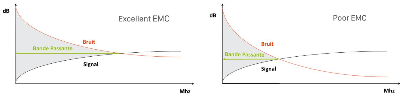
To summarize, throughput is directly related to bandwidth which is defined by noise level and, therefore, EMC immunity. The better the immunity, the closer the actual throughput will be to the theoretical throughput. As such, systems which meet EMC requirements will benefit from a lower transmission error rate and a more consistent throughput.
