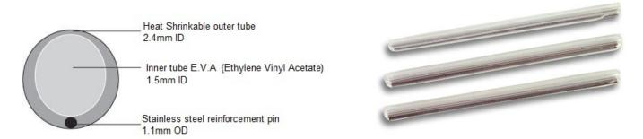
P/N: MANCHONEPISSUR60 60mm heat shrinkable splice-protectors Suitable for multimode or singlemode splice protection.
